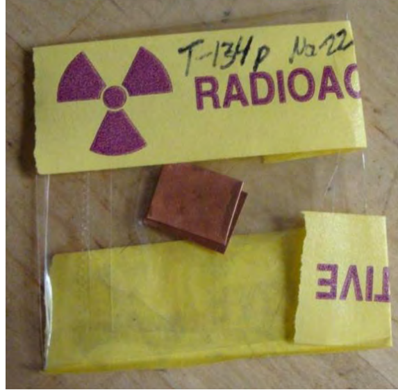
Figure 25. Picture of the copper standard source, T-134P made by Walker [29]. A similar source, T-127L, was made as a calibration and alignment source on 18 Jan 2012 with an initial activity of 23.3 \mu\text{Ci} .
