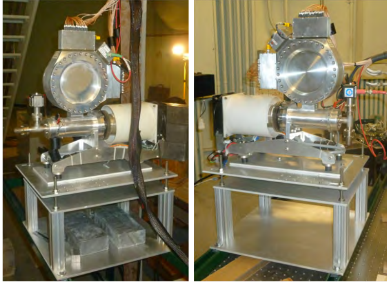
Figure 15. Pictures of the PHDs double-sided strip detectors (DSSDs) used in the three-dimensional positron annihilation spectroscopy system (3DPASS). Detector 0 is on the left and Detector 1 is on the right. Both are mounted on a 3-axis position translator designed to align the detectors to the vacuum chamber.
