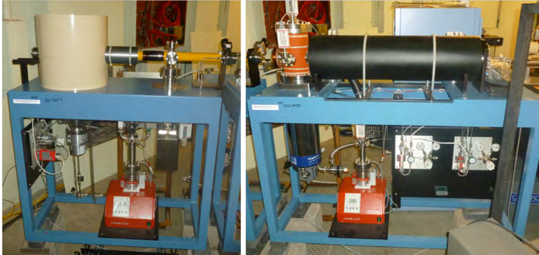
Figure 20. Picture of the First Point Scientific positron beam system at AFIT. The positron source moderator (RGM-1) is to the left, and the buffer gas positron trap (APBS) is to the right.
