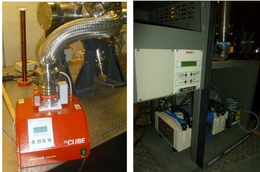
Figure 19. Pictures of the Pfeiffer HiCube 80 Eco turbo pumping station (left), Varian V-70LP turbo pumping station (right), connecting hardware, and the MDC vacuum chamber.
