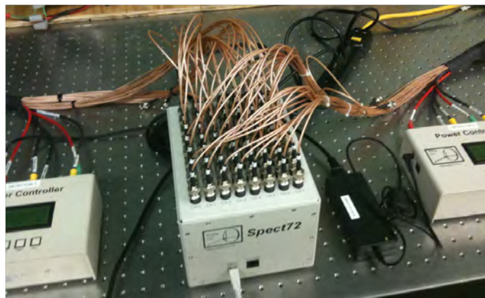
Figure 17. Picture of Spec72 digital electronics processing unit and power controllers for each detector. Each of the cables plugged into the top of the unit carries a signal from either one of the DSSD channels or one of the other detectors.
